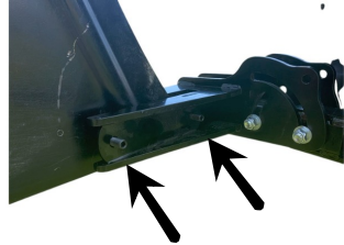
Figure 2: Universal Mounting Bracket on Bucket
